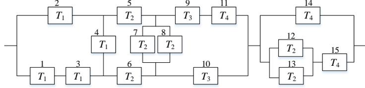
Figure 5: 15-unit structure system
